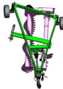
Shipping kit installed ready for truck
